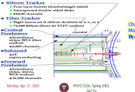
Charged Particle Momentum Resolution **D**p<sub>T</sub>/p<sub>T</sub> ~ 5% @ p<sub>T</sub> = 10 GeV/c
