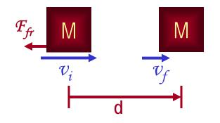
Friction force  $\mathcal{F}_{fr}$  works on the object to slow down The work on the object by the friction  $\sigma$  is
