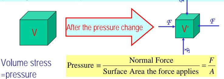
If the pressure on an object changes by  $\Delta P = \Delta F/A$ , the object will undergo a volume change  $\Delta V$ .
